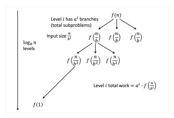
The levels of the tree range from i=0 to  $\log_b n$  with input size  $\frac{n}{b^i}$  and number of subproblems per layer  $a^i$ . Then the runtime per layer is  $a^i \cdot f\left(\frac{n}{b^{i-1}}\right)$ , or in total,
